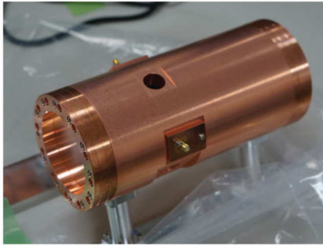
Fig. 11. Microwave cavity for zero-field experiment.
