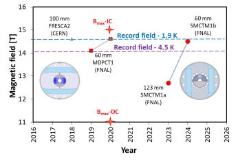
**Fig. 10.**  $B_{max}$  in the aperture and in the inner ( $B_{max}$ -IC) and outer ( $B_{max}$ -OC) coils of dipole magnet MDPCT1 and in the inner (MDP03) and outer (SMCT1) coils of the dipole mirror magnets SMCTM1a/b at 1.9 K.
