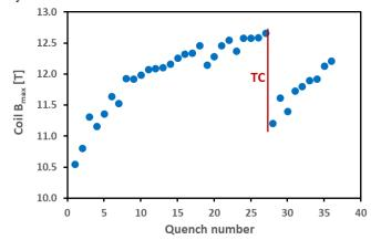
Fig. 3. SMCT1 coil  $B_{max}$  vs. quench number measured at 20 A/s and 1.9 K in SMCTM1a.
