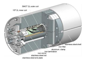
Fig. 2. 3D view of the 4-layer dipole mirror magnet.
