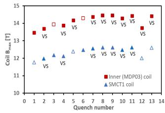
**Fig. 6.**  $B_{max}$  of MDP03 and SMCT1coils vs. quench number measured at 20 A/s and 1.9 K in the SMCTM1b. Solid markers indicate the coil where the quench originated.
