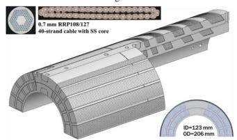
**Fig. 1.** Nb<sub>3</sub>Sn strand and cable cross-sections (top left), 3D-view (middle) and cross-section (bottom right) of the 123-mm aperture two-layer SMCT1 coil.
