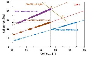
**Fig. 9.** Load lines (LLs)  $B_{max}/I$  for SMCT1 coil in 2-layer SMCTM1a and for MDP03 and SMCT1 coils in 4-layer SMCTM1b as well as expected  $I_q(B)$  curve for SMCT1 coil based on SMCT1 coil training results in SMCTM1a.
