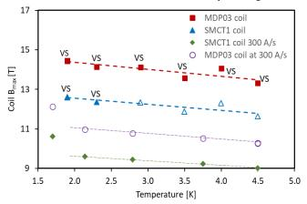
**Fig. 8.** B<sub>max</sub> of MDP03 and SMCT1 coils vs. temperature in SMCTM1b at *dl/dt* of 20 and 300 A/s. Solid markers indicate the coil where the quench originated.
