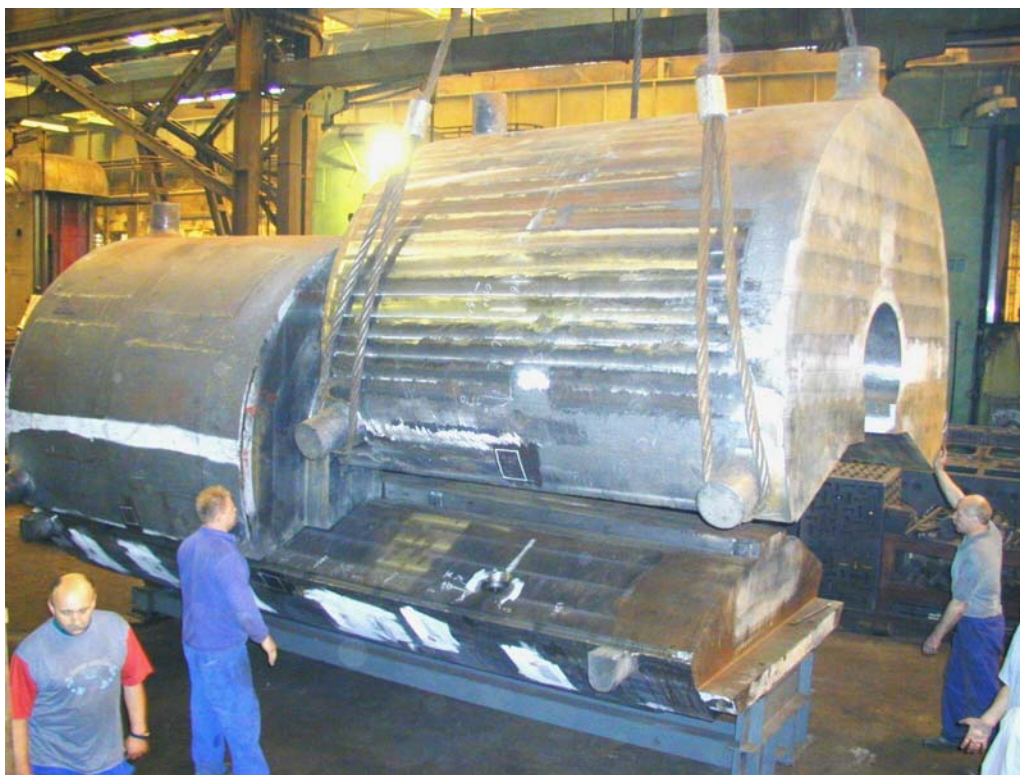
Figure 4.9 The three cast iron pieces of the JF core section during manufacturing at the Skoda factory.
