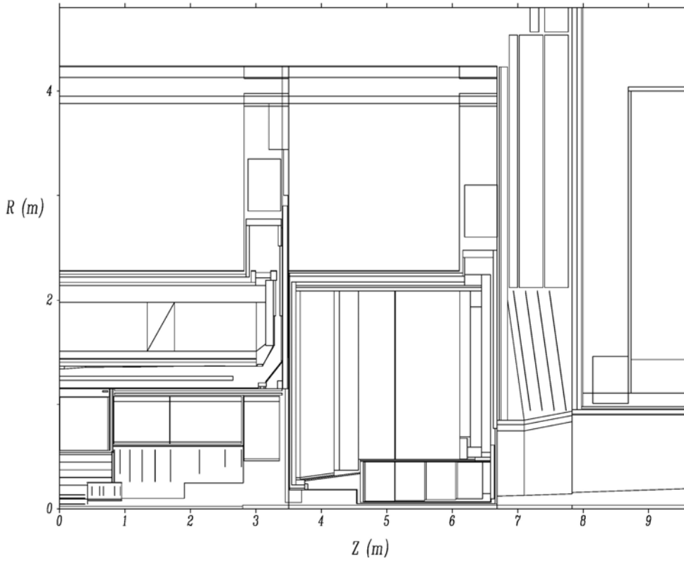
Figure 4.13 GCALOR TP43 geometry: calorimeter region.
