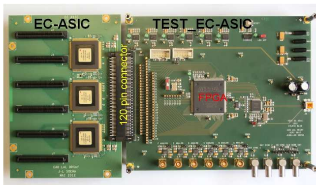
Fig. 10: Picture of the ASIC prototype board connected to a dedicated test board.
