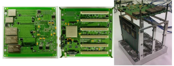
Fig. 8: Top and bottom views of PDM board (left). PDM and EC-ASIC board fixed on the mechanical structure(right).
