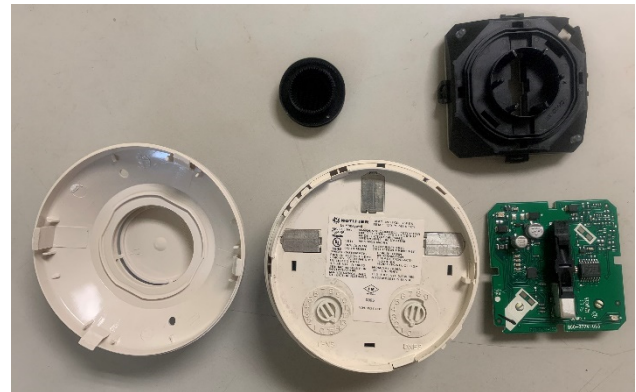
Figure 3: Visual inspection of failed smoke detectors.
