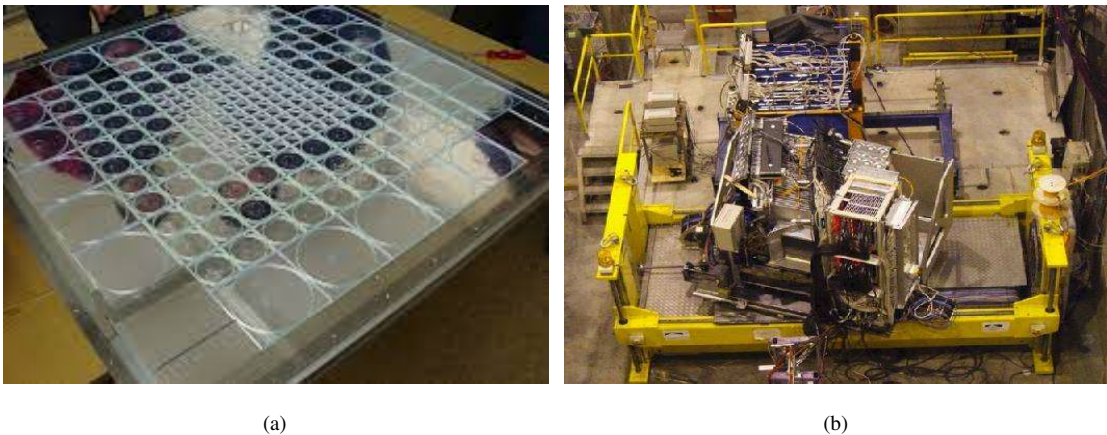
FIGURE 1.16: (a) Picture of an active layer of the AHCAL physics prototype. (b) Picture of the AHCAL physics prototype at the CERN-SPS test beam. The pictures are taken from [79].
