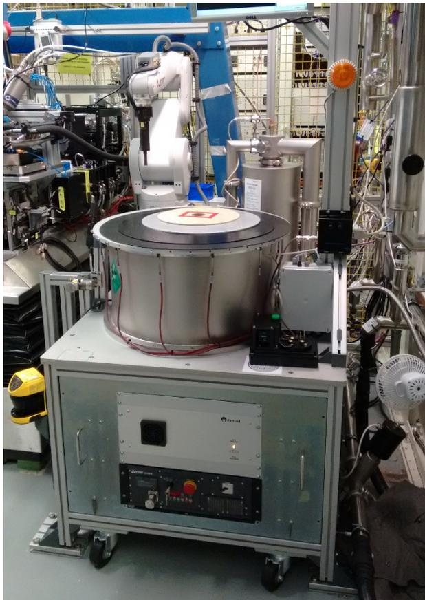
Figure 3: Complete system: Base table housing Mitsubishi controller, PLC integration unit, with laser scanner mounted on left hand side and a camera gantry and dewar with heating elements on top.
