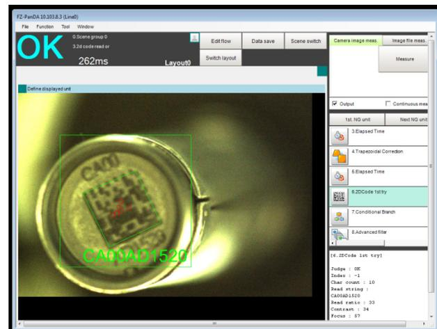
Figure 2: Screenshot of vision system reading a Data Matrix barcode.
