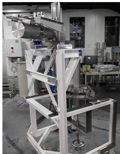
Figure 15: Cavity being lowered onto cavity-coupler assembly frame during trial assembly at RI premises.
