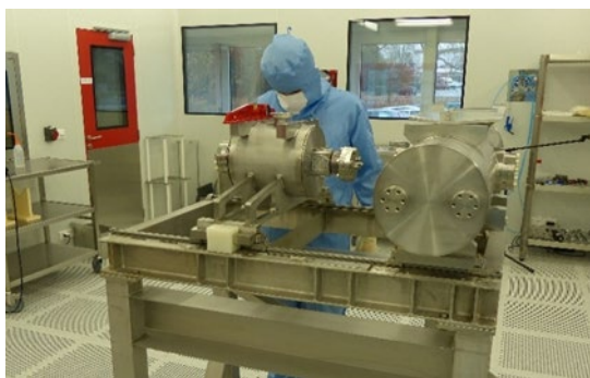
Figure 14: Trial assembly in clean room at CEA Saclay using the dummy components.
