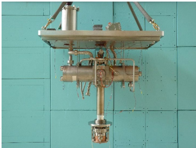
Figure 8: Cavity with its tuning system and power coupler installed on the top lid cryostat.
