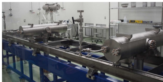
Figure 16: Start of assembly work at Rokkasho Fusion Institute. The first two cavity-coupler assemblies on the cold mass support frame, with the third cavity-coupler assembly in the background.
