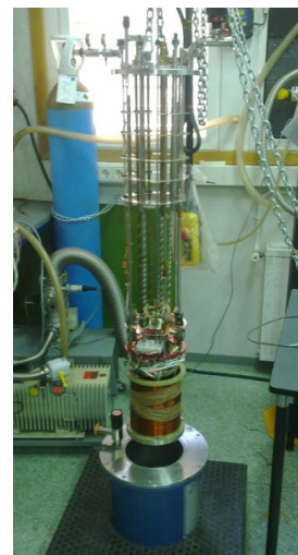
Figure 6: coils prepared for cold tests.
