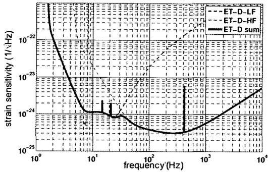
Figure 2: Xylophone design of the Einstein Telescope. The low frequency part (LF) of the sensitivity curve is realised with a low laser power interferometer operating at cryogenic temperatures while the high frequency (HF) part is covered by a room temperature interferometer with a circulating laser power of up to 3MW.
