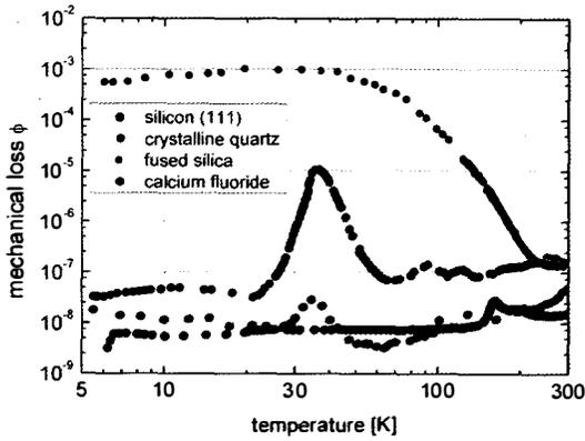
Figure 3: Comparison of the mechanical loss of different materials at low temperatures.
