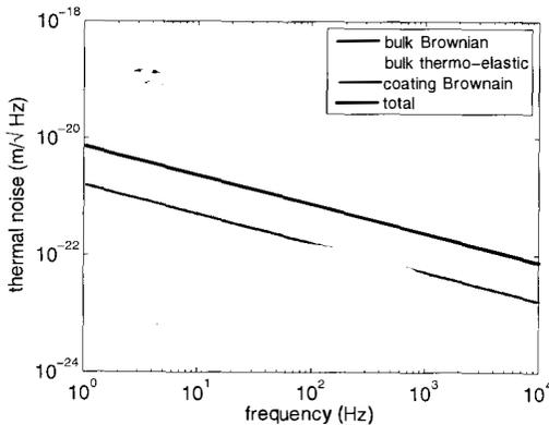
Figure 4: Summary of the thermal noise of a silicon end mirror coated with a standard tantala:silica HR multilayer.
