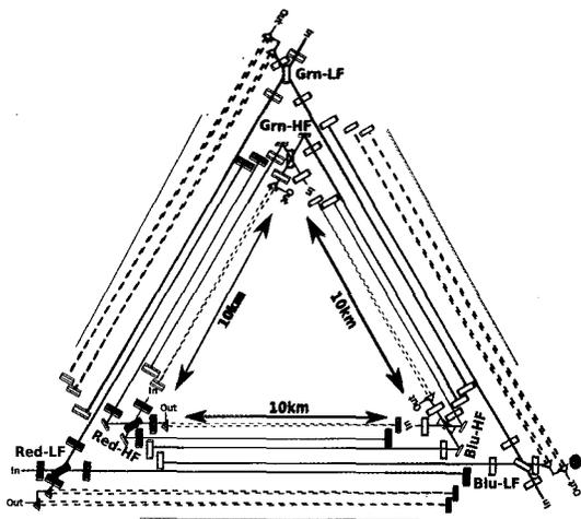
Figure 6: Triangular shape of the proposed Einstein Telescope design. Each corner station contains two interferometers - one cryogenic interferometer for the low frequency part and one high laser power interferometer for the high frequency part of the spectrum.
