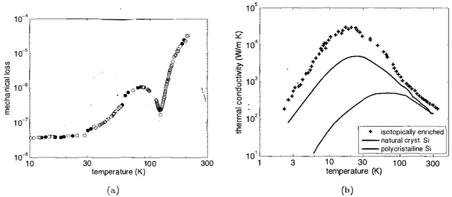
Figure 5: Mechanical loss (a) and thermal conductivity (b) of silicon as a suspension material.
