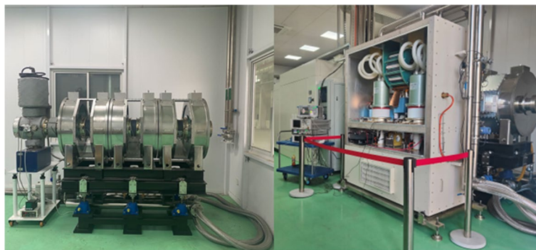
Fig. 5 Left, the magnetic alloy acceleration cavity. Right, the cavity coupled to a power source under test in a vacuum of 5.5 \times 10^{-12} Pa
