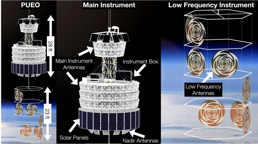
**Figure 3:** A diagram showing the PUEO instrument. Left panel: the full instrument as it will be deployed. Middle: the main instrument, including the instrument box and 108 broadband dual polarized antennas. Right panel: The Low Frequency instrument, with 8 dual-polarized broadband antennas.
