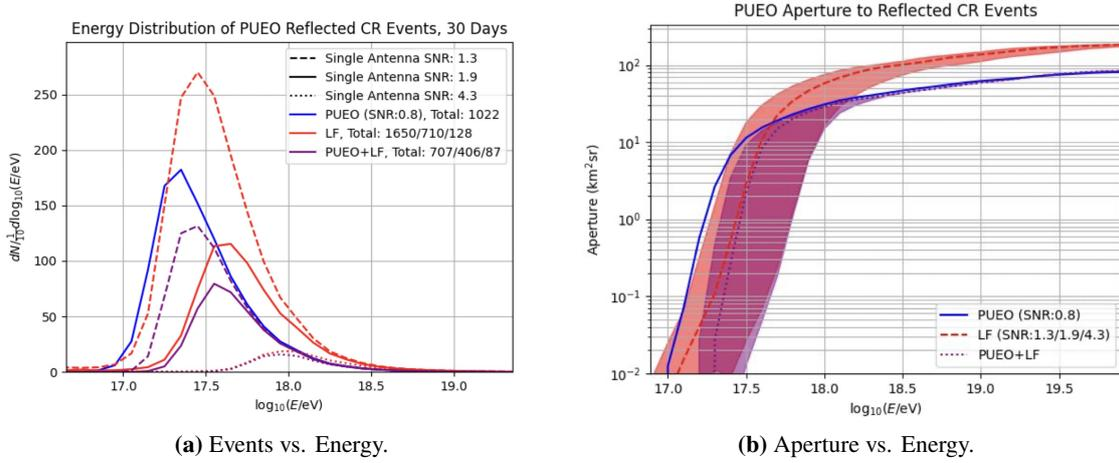
**Figure 5:** Left: the number of reflected cosmic ray events seen by each of PUEO’s instruments as a function of primary energy. The different line styles are three possible thresholds for the LF instrument. Right: The aperture of the PUEO instruments as a function of reflected cosmic ray energy.
