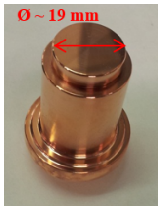
Figure 3.2: Picture of the CERN copper substrate
