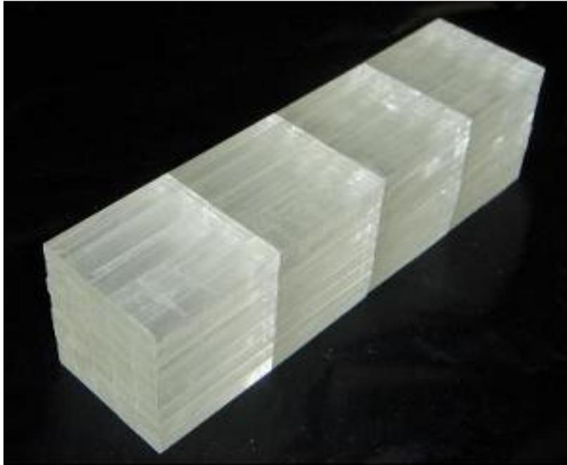
Figure 16.2: Photograph of stacked crystals for a prototype electron calorimeter composed of 160 GSO(Ce) crystals of  $4 \times 6 \times 30 \text{ mm}^3$ .
