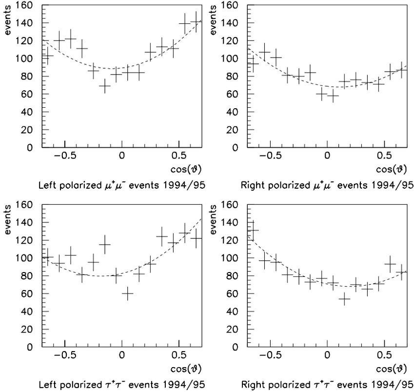
Figure 2: Polar angle distribution for  $Z$  decays to muons and taus for the 1994-5 SLD run. The left column shows the distributions for left beam polarization; events produced with the right beam polarization are on the right. The excess of events in the left plots illustrates  $A_{LR}$ . The difference in forward backward asymmetries for the left and right plots allows extraction of the final state lepton coupling parameter.
