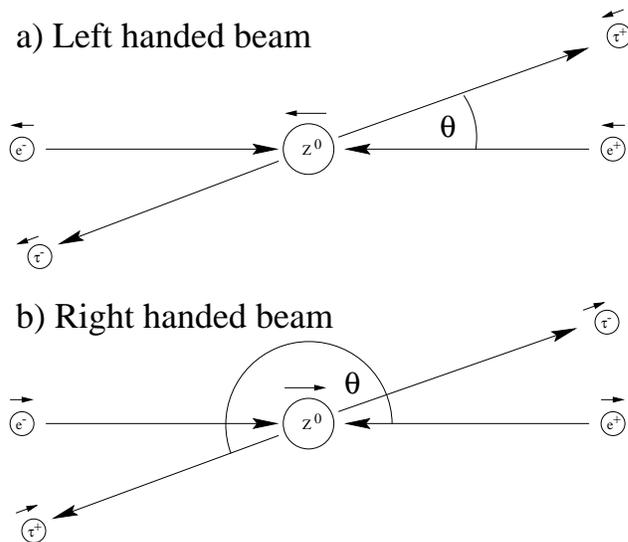
Figure 1: Electron helicities in  $Z$  production. a) shows the Left cross section and b) the Right cross section. Long arrows represent the lepton momentum; short arrows indicate the longitudinal spin projections.
