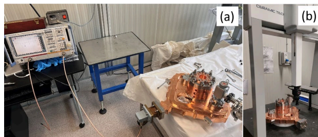
Figure 5: (a) RF Tests of The Gun; (b) Mechanical Characterization of the Gun With CMC.
