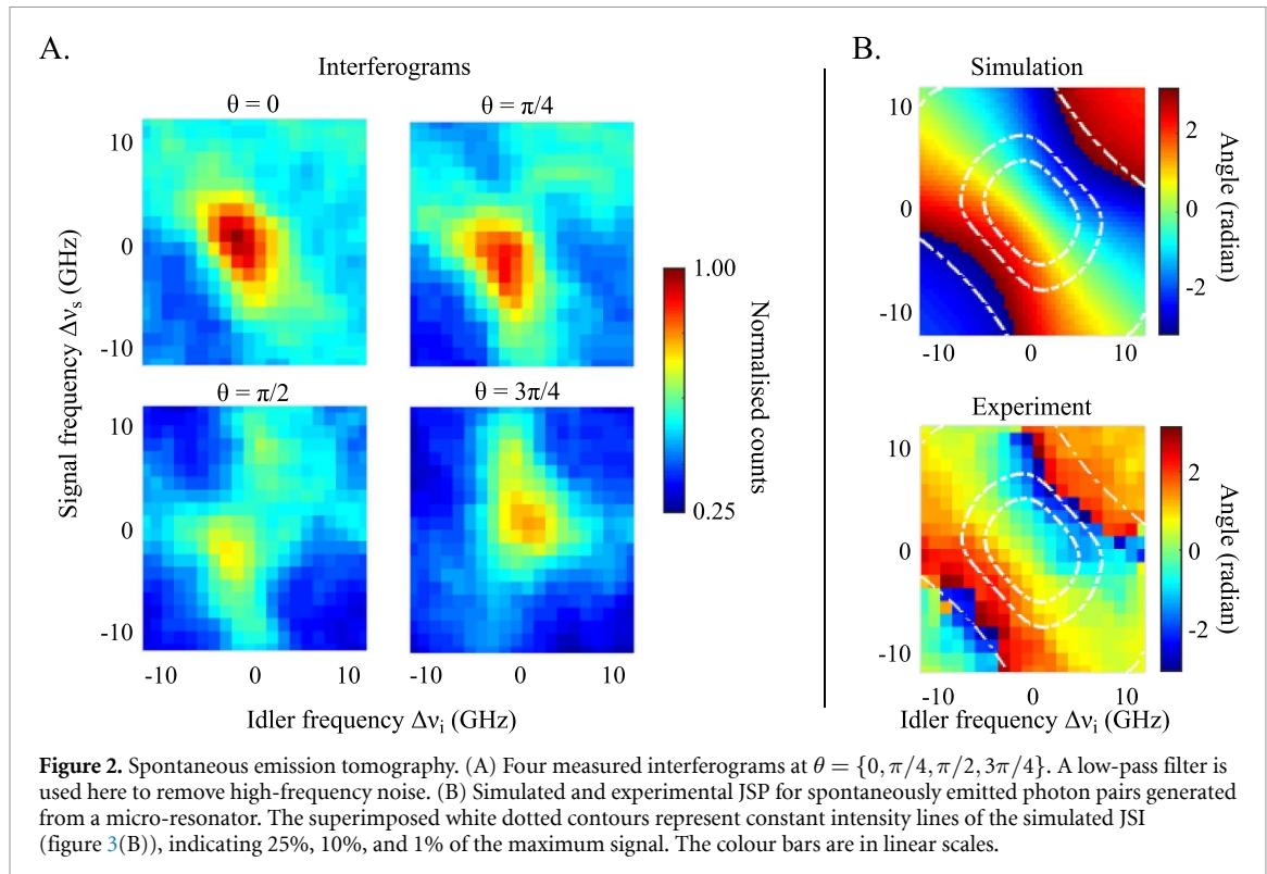
**Figure 2.** Spontaneous emission tomography. (A) Four measured interferograms at  $\theta = \{0, \pi/4, \pi/2, 3\pi/4\}$ . A low-pass filter is used here to remove high-frequency noise. (B) Simulated and experimental JSP for spontaneously emitted photon pairs generated from a micro-resonator. The superimposed white dotted contours represent constant intensity lines of the simulated JSI (figure 3(B)), indicating 25%, 10%, and 1% of the maximum signal. The colour bars are in linear scales.
