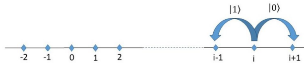
Fig. 1. Illustration of a discrete-time quantum walk on a one-dimensional lattice. At each time step, a quantum coin determines the walker’s direction: outcome |0\rangle results in a rightward move from position i to i + 1 , while outcome |1\rangle causes a leftward move from i to i - 1 .
