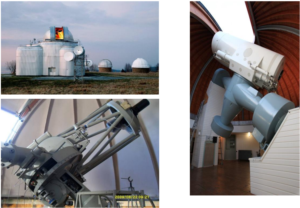
Fig5. Small SAO's telescopes. Top left: general view of the domes. Right: the 1-meter telescope Zeiss-1000. Bottom left: the 60-cm telescope.
