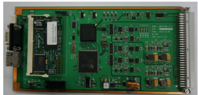
Figure 1: DSP Board that includes DSP, FPGA, ADCs and the other components.
