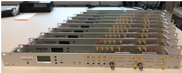
Figure 2: ESS production of two arc detectors with 1 lux sensitivity, 850 ns reaction time, false trigger filtering, on board full optical path test function, adjustable gain and analogue output monitoring, network connection and HMI.
