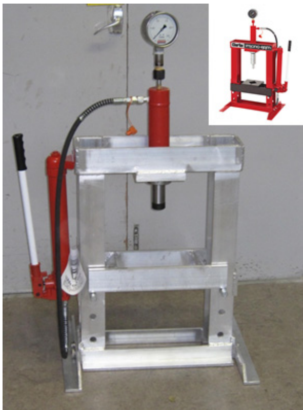
Figure 2: Press for frequency measurements of dumb-bells and half-cells.
