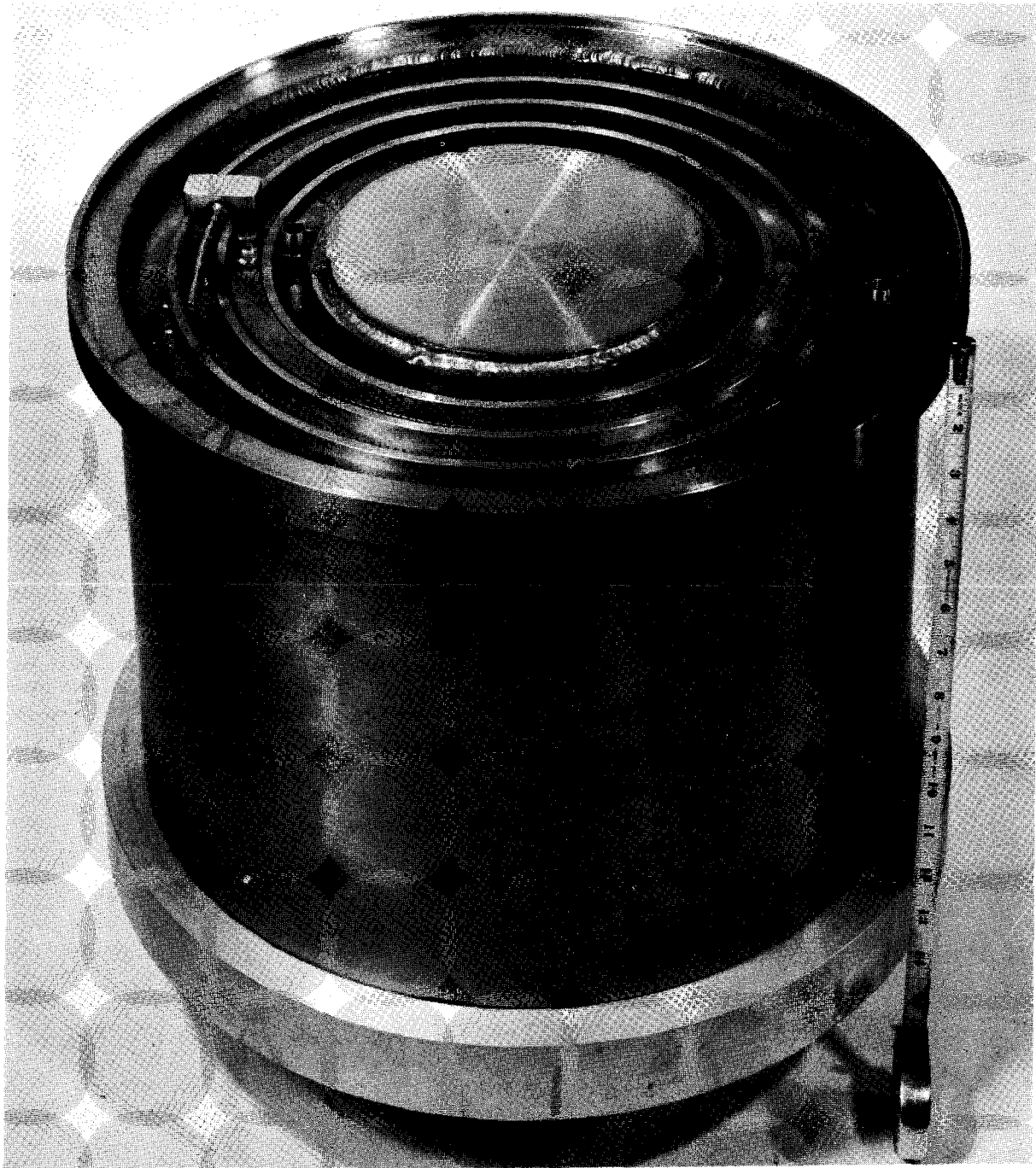
Fig. 2 Mold for coil of 8-inch inside diameter; sodium has not yet been cast in place.
