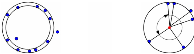
Figure 4. Illustration of the narrow corridor around the ring (left) and the angles between neighboring hits (right).
