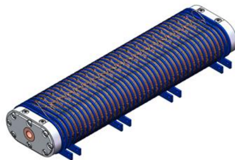
Figure 6: MgB2 undulator magnet half. Magnet core consists of a copper conductive cooling rod, 1006 carbon steel magnet core, vanadium permendur yokes (colored in blue for clarity), and the main coil
