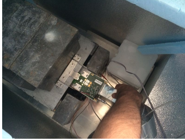
Figure 3.6: Photograph of the experimental setup used for the measurement of charge collection of miniature sensors. It includes the Alibava readout bonded to the sensor and the lead enclosure under which the strontium-90 source, scintillator, and photomultiplier tube are located.
