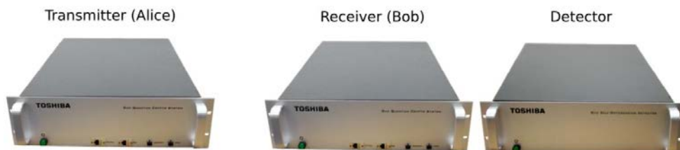
Fig. 1. Photograph of the prototype high speed QKD system. The transmitter (Alice) is connected to the receiver (Bob, which includes a separate detector unit) by a pair of telecom fibres (not shown); the first fibre is used for quantum signals and the second fibre for classical communication.
