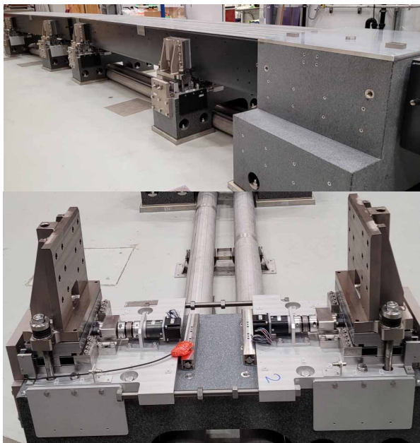
Figure 3: Pictures of half arc girders (top) and of the girder adjustment system (bottom).
