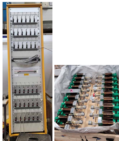
Figure 5: Five amperes PS racks with 36 units (left) last batch of X-Y corrector pairs (right).
