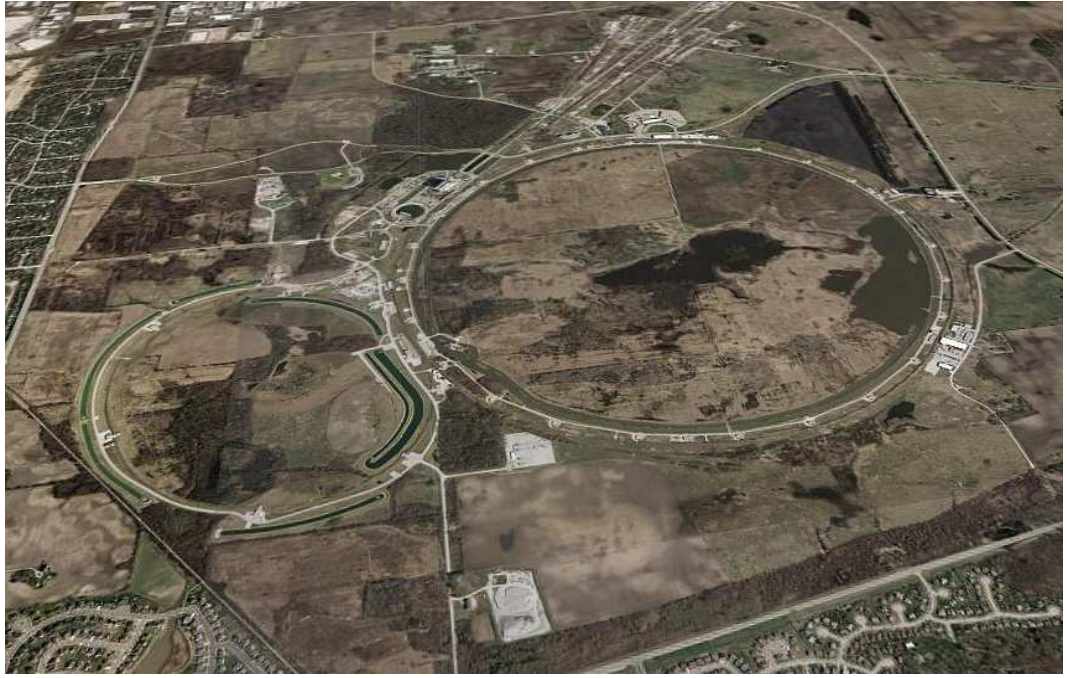
Figure 3.1. Four miles in circumference, the Tevatron p\bar{p} collider is housed in a tunnel about 30 feet below the big ring you see in this aerial view of the Fermilab. The ring to the left of it is the Main Injector. Photo is courtesy of Google Earth™.
