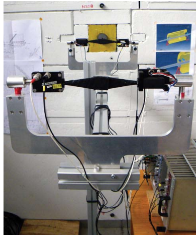
Fig. 7.10: The coincidence signal of two overlapping pairs of scintillators, in front of the setup, is used as trigger signal.
