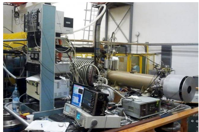
Figure 2: Krion-6T at high-voltage platform of LU-20 fore-injector.
