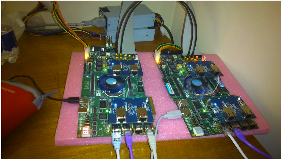
Figure 3.19. Test bench environment. Two DE4 boards connected together. One with the L0TP firmware, while the other runs the firmware to emulate the environment surrounding the L0TP.
