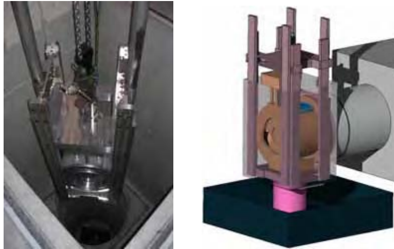
Figure 9: n_TOF new spallation target assembly being lowered in the pit (left); geometrical FLUKA implementation of the new target assembly inside the old container (right) [4]
