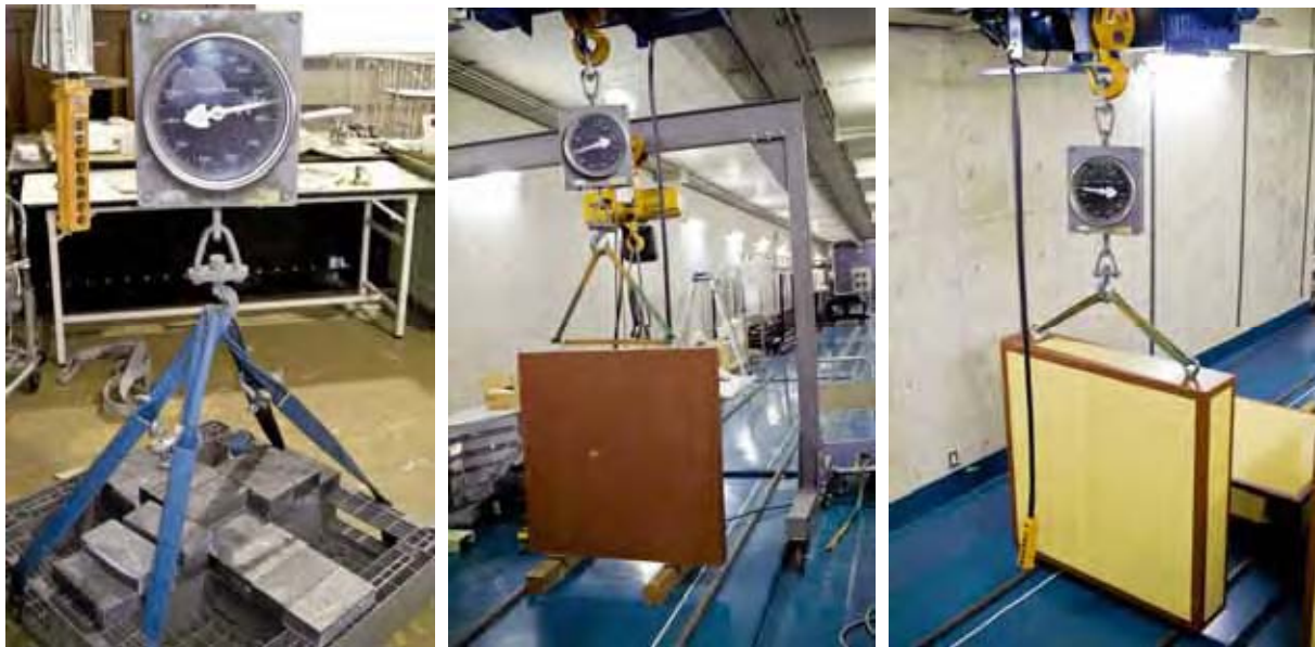
Figure A1: Calibration by lead and density measurement of iron and concrete shields
