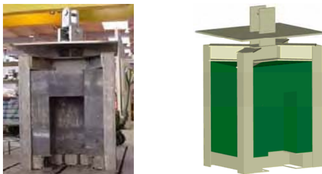
Figure 2: First n_TOF lead target (left) compared to the geometrical FLUKA implementation (right) [4]
