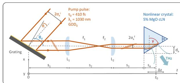
Figure 1: Schematic drawing of the setup including crucial tuning parameters.
