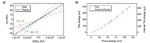
Figure 3: (a) The relative position of the crystal for maximum efficiency vs.  $GDD_0$  on the pulse match the position computed for the temporal focus. (b) THz energy extracted from a setup pumped with stretched pump pulses ( $GDD_0 = 1.44 \text{ ps}^2$ ).
