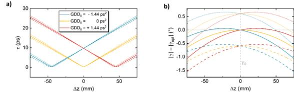
Figure 2: (a) Pulse duration vs  $\Delta z$  for initially compressed (yellow) and stretched (blue, red) pump pulses. Dashed ( $\theta_d^{\text{opt}} + 1^\circ$ ) and dotted lines ( $\theta_d^{\text{opt}} - 1^\circ$ ) show the effect of  $\theta_d$ . (b) The corresponding pulse-front tilt  $\gamma$  vs.  $\Delta z$ .
