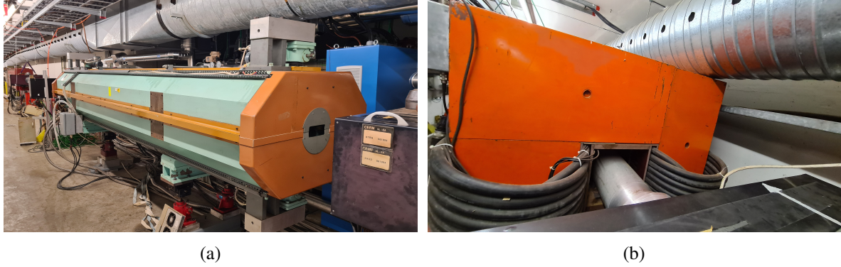
Figure 2.12: The two types of magnetic collimators used in the M2 beamline. Fig. 2.12(a) highlights the scraper magnet. Those are 5 m long and have a movable aperture. Fig. 2.12(b) shows a magnetised iron block, which is 1.6 m long with a beam pipe of 200 mm diameter. Both magnetic collimators provide a toroidal field of the order of 1 T.
