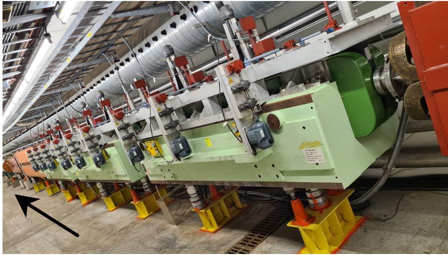
Figure 2.19: Photo of the absorber section in M2. The black arrow indicates the beam direction. Each magnet is 3 m long.
