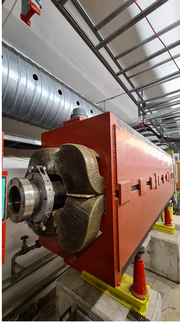
Figure 2.8: Picture of a quadrupole magnet of type Quadrupole West Area Long QWL installed in the M2 line. It is 2.948 m long with a beam pipe of 100 mm diameter.
