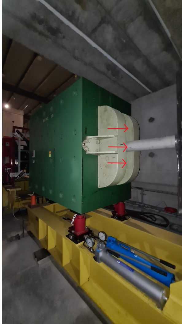
Figure 2.6: Picture of a vertical dipole magnet installed in the M2 line. The arrows indicate the magnetic field lines. The good field region is not to scale; in reality, it is smaller. The magnet is 2 m long with a full aperture of 192 mm \times 140 mm.
