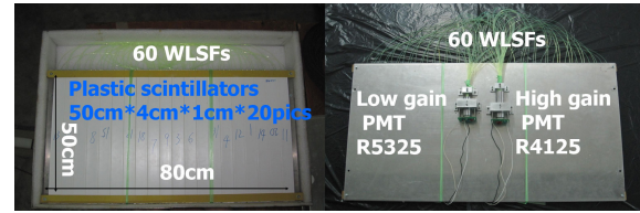
Fig. 19. The outlook of YAC detector. Each YAC detector consists of a scintillator of 80 cm × 50 cm in area with 1 cm thickness and lead absorber of 3.5 cm thickness above the scintillator. Such design provides geometrical uniformity of the detector response within \pm 6\% . A couple of PMTs are used to cover wide dynamic range of the number of particles (burst size) from 1 MIP to 10 6 MIPs.
