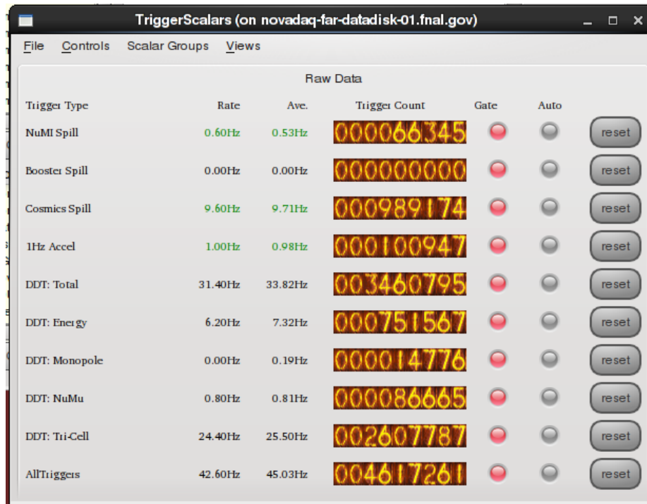
Figure 4.2: The Trigger Scalars, showing the total number of triggers issued, broken down by type, with a DDT subtotal and an overall total.
