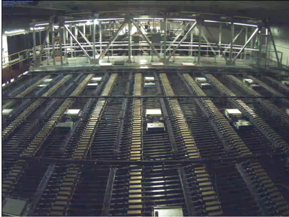
Figure 3.7: View of the top of the FD , the electronics boxes for the first three diblocks can be seen
