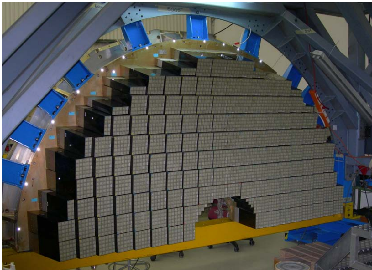
Figure 2.11: An endcap Dee. A Dee is half of one endcap. The crystals are grouped in units of 5 \times 5 crystals called supercrystals. [53].
