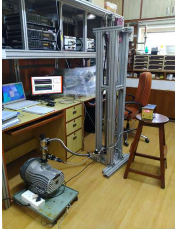
Figure 2.13: Initial vacuum test of the probe lift.
