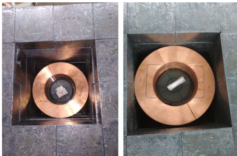
Figure 5.2: Pictures showing the typical sample mounting arrangement for samples in TiLES (close geometry).
