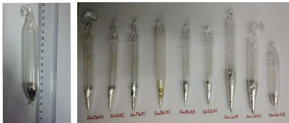
Figure 3.2: Selected pictures of samples that were synthesized. Left: 7N pure Sn single crystal grown using vertical Bridgman technique; Right: A set of Sn-rich alloy samples grown in a box furnace under identical conditions.
