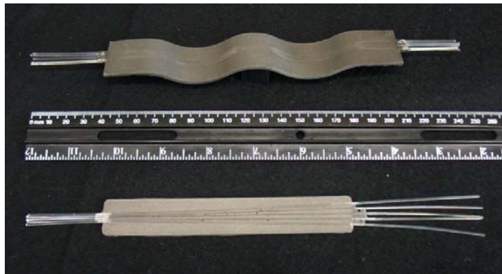
Figure 5. Accordion layer (top) containing tungsten powder epoxy and embedded scintillating fibers.
