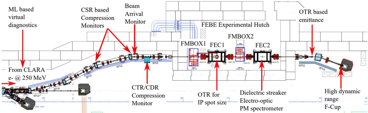
Figure 1: Engineering diagram of FEBE beamline, highlighting areas with diagnostic systems undergoing R&D. These areas are supported by diagnostic systems including Ce:YAG screens, beam position monitors and ICTs.
