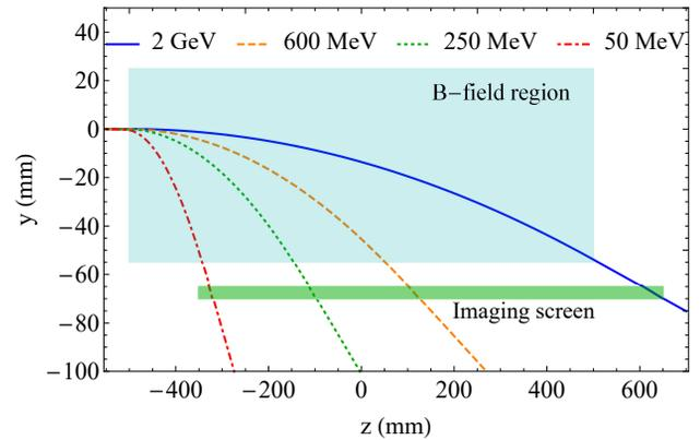
Figure 2: The physical extent of the full PM dipole system for use in FEC2, along with imaging screen. Electron trajectories for the full operating range are shown.
