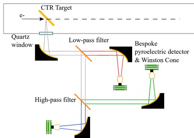
Figure 4: Schematic diagram of the BCM spectrometer system to be installed at end of FEBE arc as indicated in Fig. 1.
