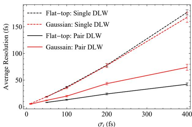
Figure 3: Simulated average resolution of a DWA streaking measurement in FEC2 for varying bunch length  $\sigma_t$  for both Gaussian and flat-top profiles (where flat-top has total length  $4\sigma_t$ ), for charge of 250 pC. The improvement in resolution from using a pair of orthogonally orientated structures to cancel higher order wakefields is shown.
