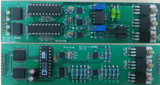
Figure 2: ADC daughter boards for current and voltage for feedback control (upper) and general purpose (lower).
