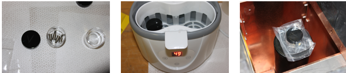
Figure 4. (Left) Four source capsules after cryogenic exposition in a water container. (Middle) Water container in a controlled temperature environment. (Right) Water container on top of a germanium low-background counter.
