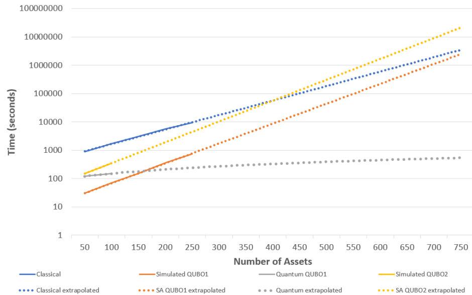
Figure 7. The computation times to solve the problems as a function of the number of assets in the portfolio. The solid lines are the results of experiments, the dotted lines are trend-lines, based on an exponential extrapolation for the classical methods and linear extrapolation for the quantum approach.
