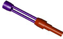
Figure 2: The FLUKA simulation model of the Tungsten collimator from the COMET cyclotron.
