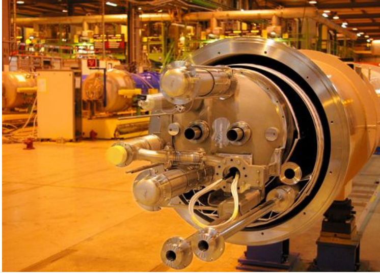
Figure 2.2: Inner structure of a dipole magnet. The two holes in the center are the beam pipes. LHC uses 1232 of these 15-meter long dipole magnets, responsible for the bending of the proton beams.
