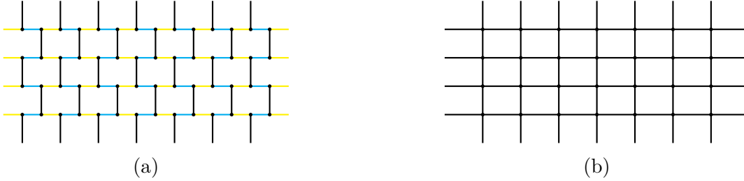
Figure 3.6. (a) Shows a honeycomb lattice where all vertices have been paired and shrunk by dominating the yellow edges. (b) The resulting effective or shrunk lattice where a toric code Hamiltonian acts.
