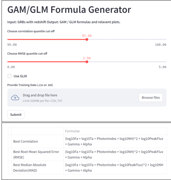
Fig. 7. Image of the GAM and GLM Formula Generator page of the web app. This module allows users to access the best formula for predicting redshift based on the training set provided and its predictors. The user can also manually set the cutoff for the correlation and RMSE in order to select the formula.
