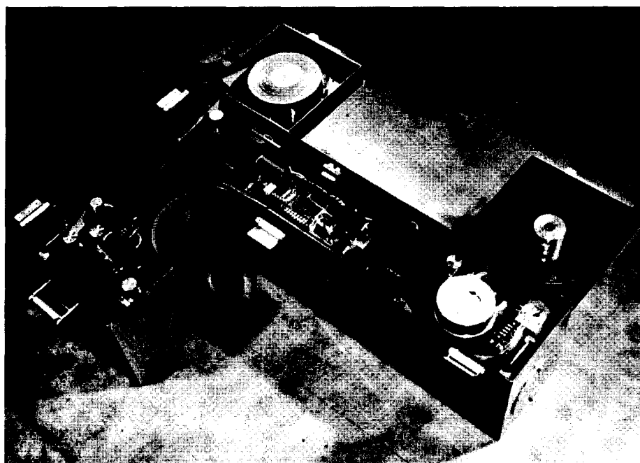
Fig. 11 The camera. The camera has three lenses, which all image on the same 46 mm film.
