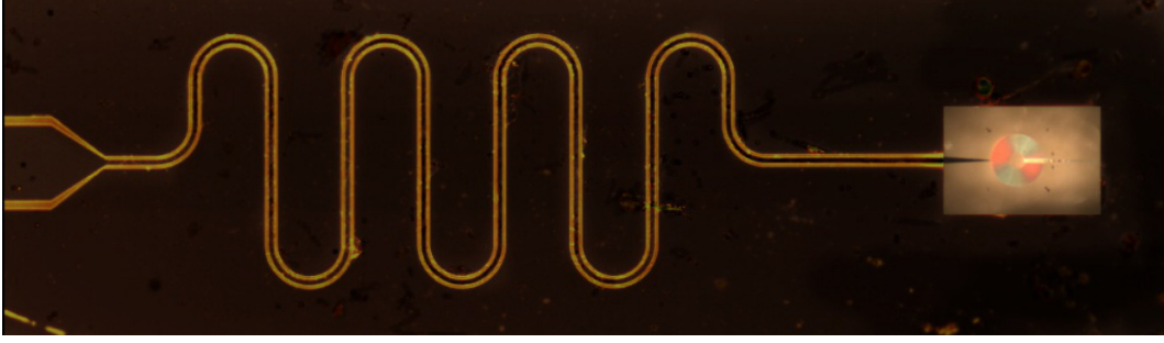
Figure 3.10: Optical image of the whole 3 mm×10 mm chip, showing the impedance adaptation resonator (meanders in the middle) and the bonding pad on the left (taken from [35]).
