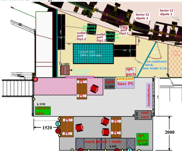
Figure 2: Scheme of the VSR Diagnostic Platform.
