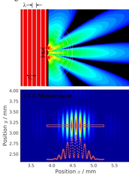
Figure 3: Transverse Interferometry: calculated double-slit interference pattern (upper plot) and CCD pattern taken at a diagnostics test beamline (lower plot).
