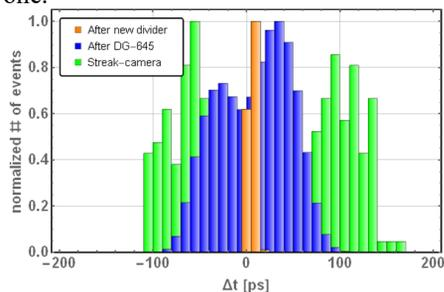
Figure 6: Long-time investigation (over about 24 hours) of the jitter in the horizontal FSC trigger systems.
