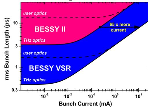
Figure 1: Comparison of standard user optics as well as THz optics for BESSY II with the future BESSY-VSR system, considering realistic SRF boundary conditions.
