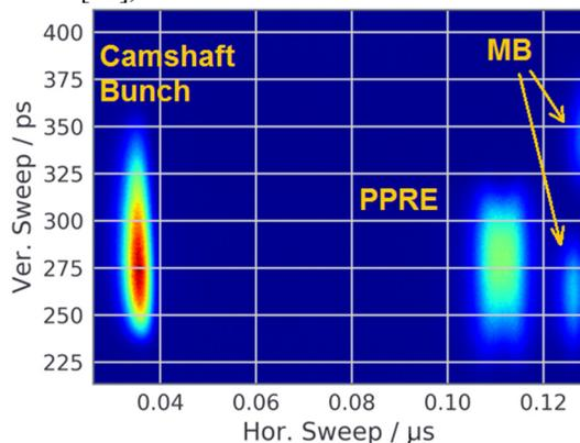
Figure 5: FSC measurement, showing the 2D time- and horizontal-size- variation for different bunch types.
