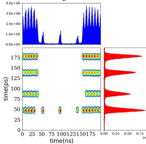
Figure 4: FSC data of the BESSY II low- $\alpha$  mode for the central 200 ns out of 800 ns bunch-fill pattern.
